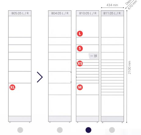
Cleveron 301 has a modular column system that allows to choose the best drawer/door configuration and layout for the APM
